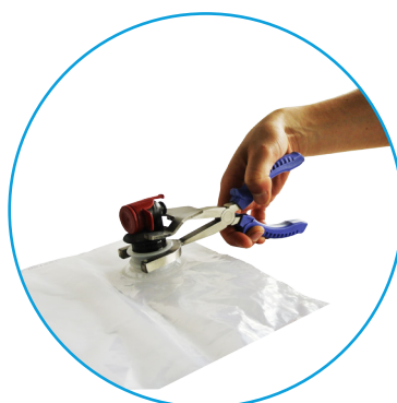
Insert the hand tool clamp in the upper part of the gland
